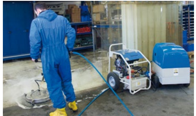
DYNAJET 350 bar and hot water used in workshop floor cleaning
